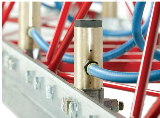
Piston vibrators on 30" centers provide 11,000 VPM to ensure maximum concrete consolidation up to 12" deep.
