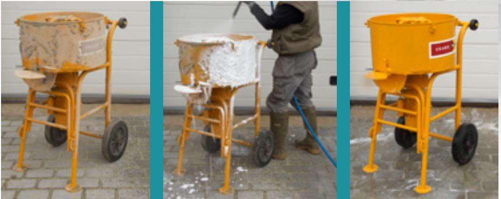
To clean off the item use a high-pressure cleaner or with water and a stiff brush. In cases where there is heavy build-up, the treatment can be repeated.
