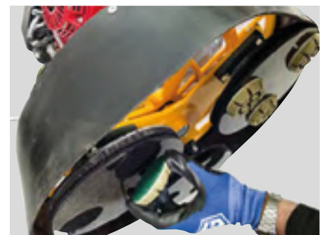
Semi-rigid plate with velcro tool attachment.
