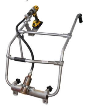
This Multivibe was tested with a DeWalt hammer drill in drill code (DCD996). The 20V battery did two loads of concrete with still half of battery life left. Each battery should give over an hour of continuous use. The drill has 3 speeds for the drill mode, speed 1 use only to chuck up to spline or to take off from screed. Speed 2- use the majority of the time and will run a Multivibe screed bar up to 12ft Speed 3 should only be used when needing extra vibration in very low slump concrete.
