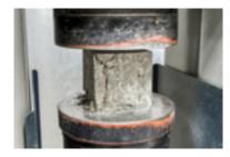
Crush the cubes to test their strength – When each cube is ready for testing, it is put into a concrete crusher. This machine exerts force onto the cube until it breaks. The rate at which it crushes is measured, and this is its compressive strength.
