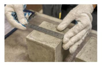
Steel or plastic concrete test moulds are used to to contain the concrete and create the cubes. These can be purchased from Speedcretes online shop.
